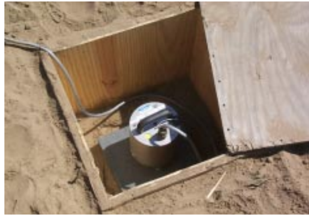
Figure 1. Seismometer in pit at site 2.
